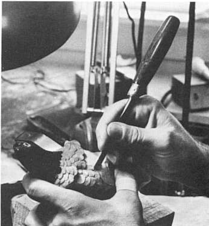
For fine carving—defining and undercutting the feathers and other features—he uses a skew chisel and holds it much as you would a pen- cil. This grip affords little power but maximum control.
