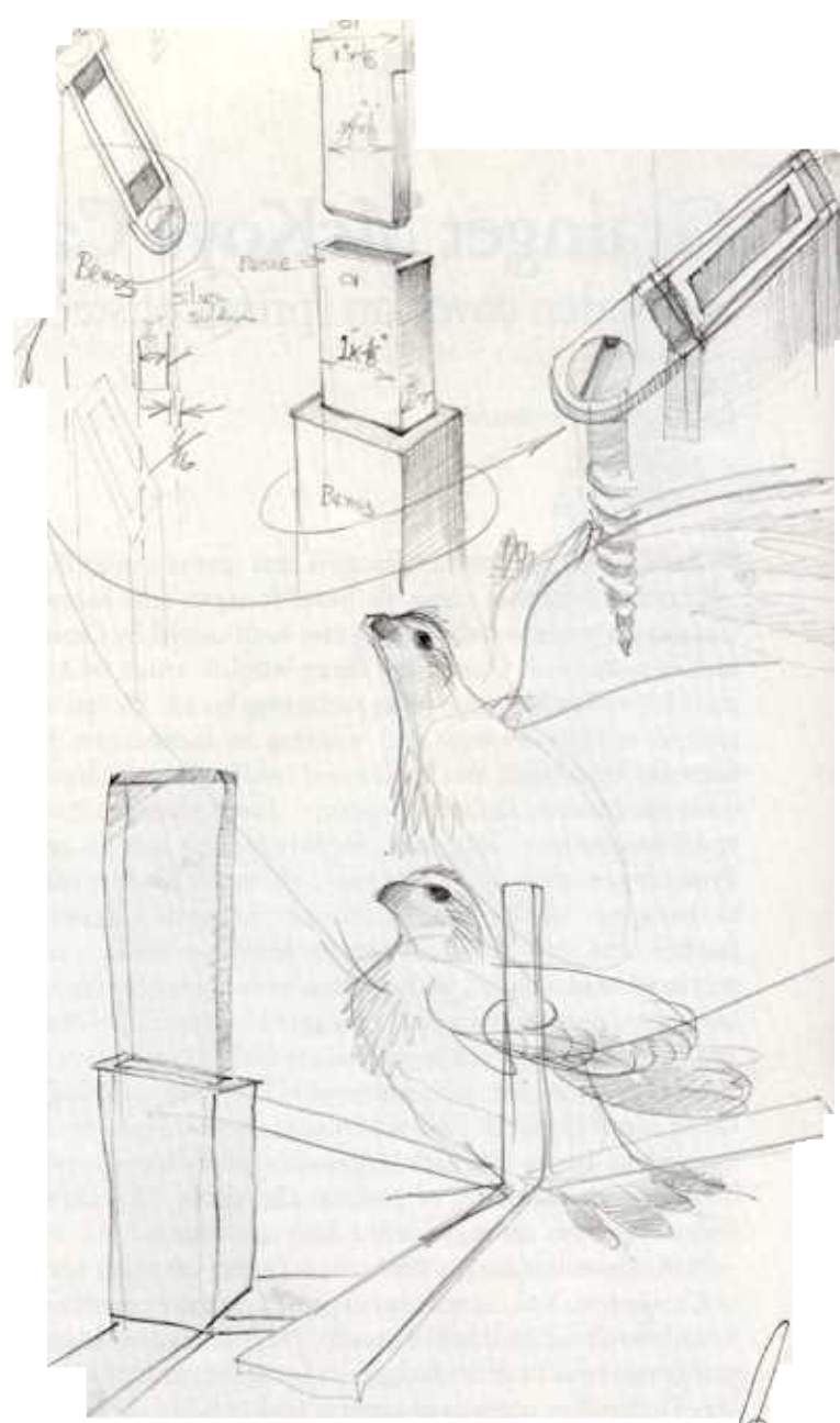
To make the bodies of the birds in his sculpture as light and structurally stable as possible, McKoy bandsaws them in two and hollows out the insides with a gouge (photo, top). Note the high-carbon steel ribbon that has been let into the wing and screwed in place. This is part of the understructure of the covey that supports the birds imperceptibly, presenting the illusion of flight. McKoy devised a tenon-and-socket joint (above) which allows the pieces to be disconnected when necessary. The basic joinery was worked out in sketches as at right.
