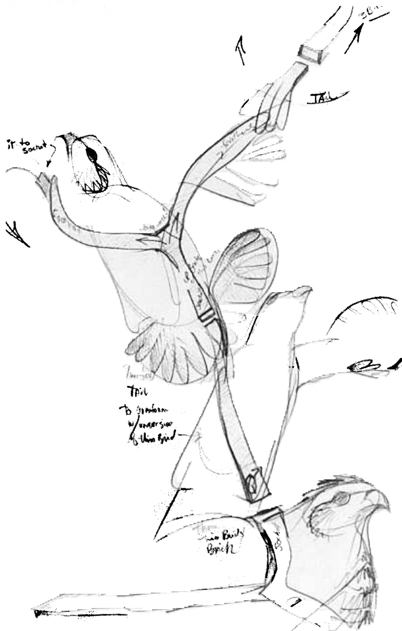
One of McKoy's preliminary sketches of his covey sculpture, showing the steel-ribbon understructure that supports each bird.
